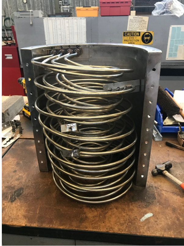
Figure 18. Brace around Heat Exchanger Coils 1
