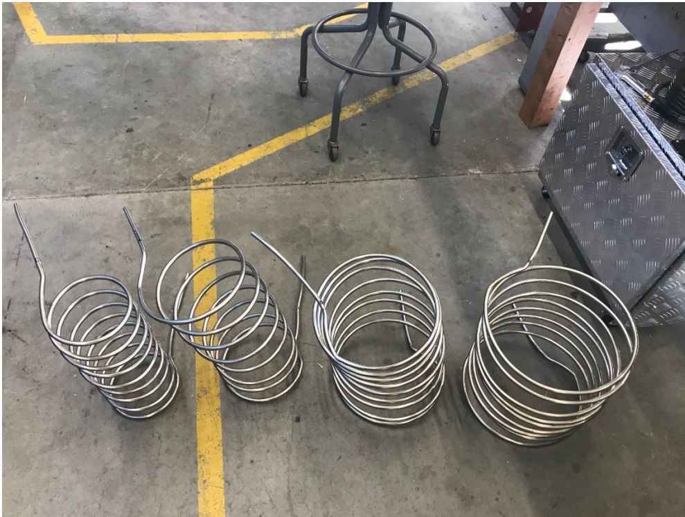
Figure 15. Heat Exchanger Coils
