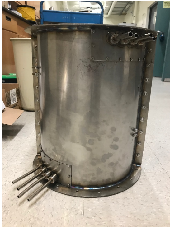
Figure 20. Assembled Heat Exchanger 1
