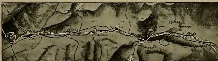
FIG. 39A.—Loop Tunnels of St. Gothard. Approach to the Great Tunnel from the South.
