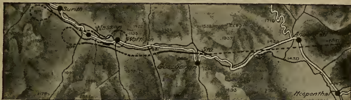
FIG. 39.—Loop Tunnels of St. Gothard. Approach to the Great Tunnel from the North.
