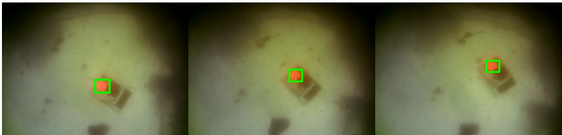
Figure 6-21: A video stream from the buoy while tracking underwater in the Charles River. Each image is 10 frames later than the previous image. Depth of 36" with LED at 100% intensity.
