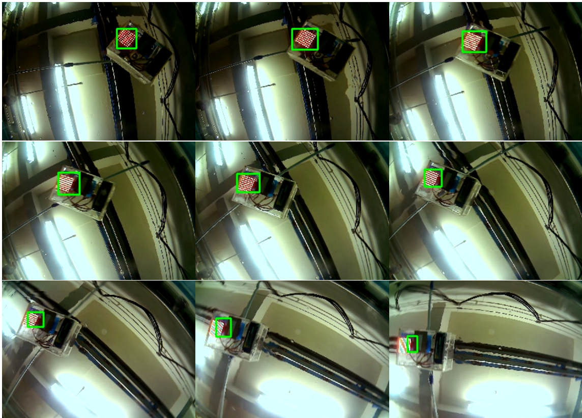
Figure 6-2: A video stream from the buoy while tracking underwater in the Tow Tank. Each image is 10 frames later than the previous image.
