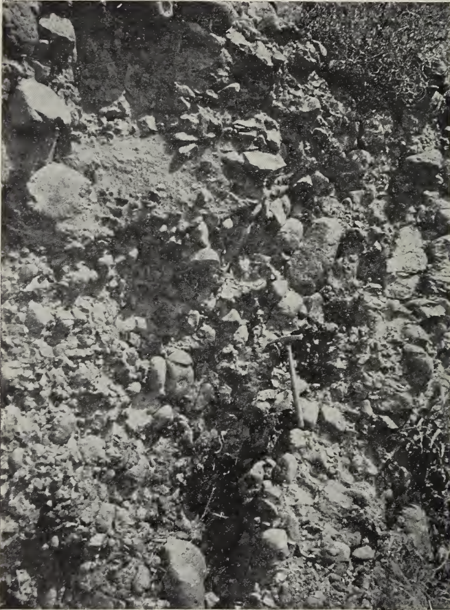
Bed of Cretaceous conglomerate on Ash Creek, Pinal County, Arizona. Andesitic tuff matrix. Dip 70 degrees to left. Boulders fractured.
