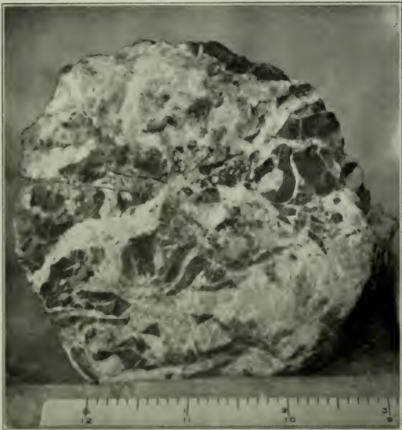
Plate IV.—Breccia in crushed mineralized zone in mine of Federal Zinc and Lead Co.
