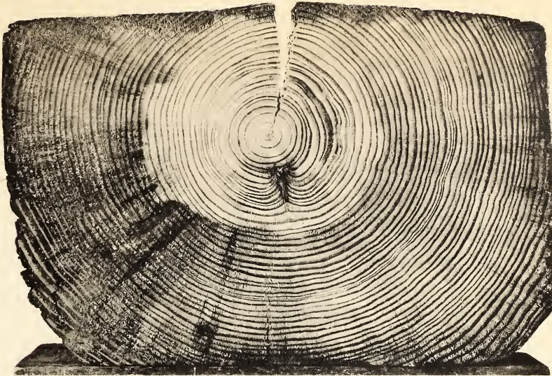
Fig. 1. New Baltic pine tie from Prussian railway, treated with chloride of zinc and tar oil.
