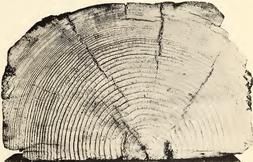
Fig. 2. Baltic pine tie laid in Prussia (Marschbahn) in 1885, treated with chloride of zinc and tar oil.
