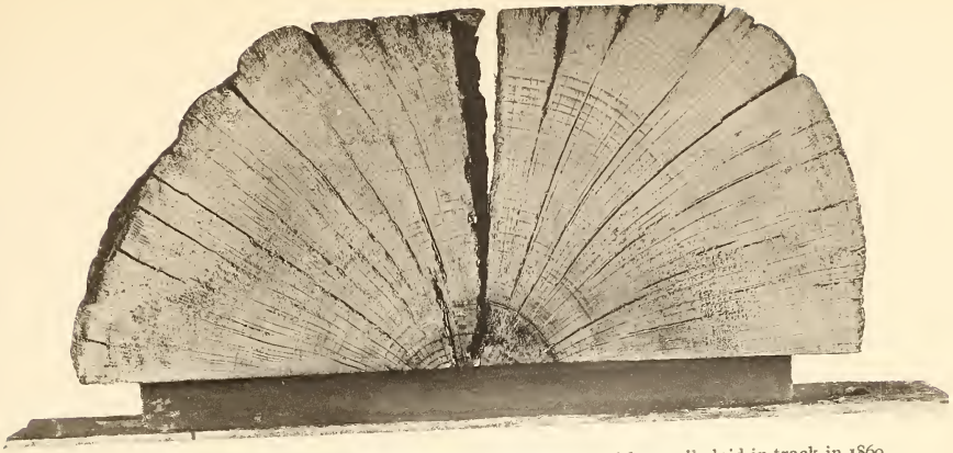
Fig. 1. Median section of beech tie (France), impregnated with tar oil; laid in track in 1869.
