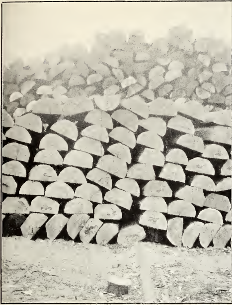
FIG. 1.—PILE OF NEW OAK TIES AT GHENT, BELGIUM. (NOTE "S" IN ENDS.)
