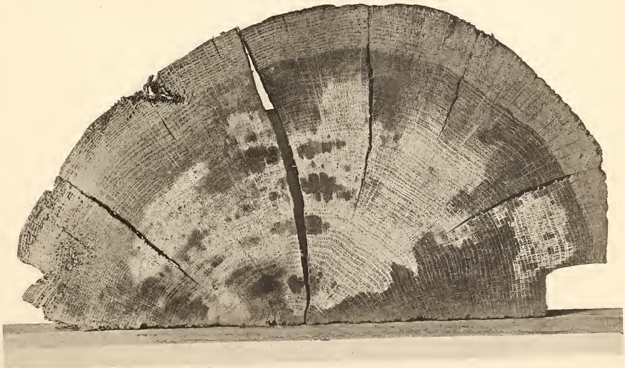
Fig. 3. End section of freshly impregnated oak tie (Belgium), using tar oil.
