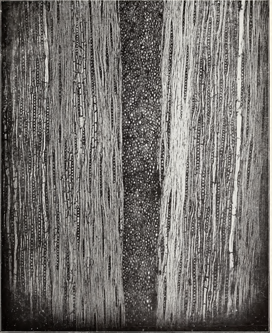
TANGENTIAL SECTION OF WOOD OF WHITE OAK.
