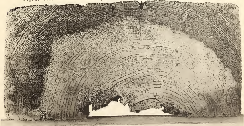
Fig. 3. Median section of Baltic pine tie, impregnated with tar oil, showing how decay starts. (This tie is still good for several years.)
