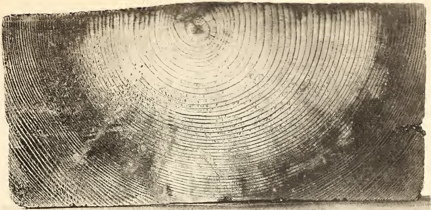
Fig. 1. Median section of new Baltic pine tie (England), impregnated with tar oil.
