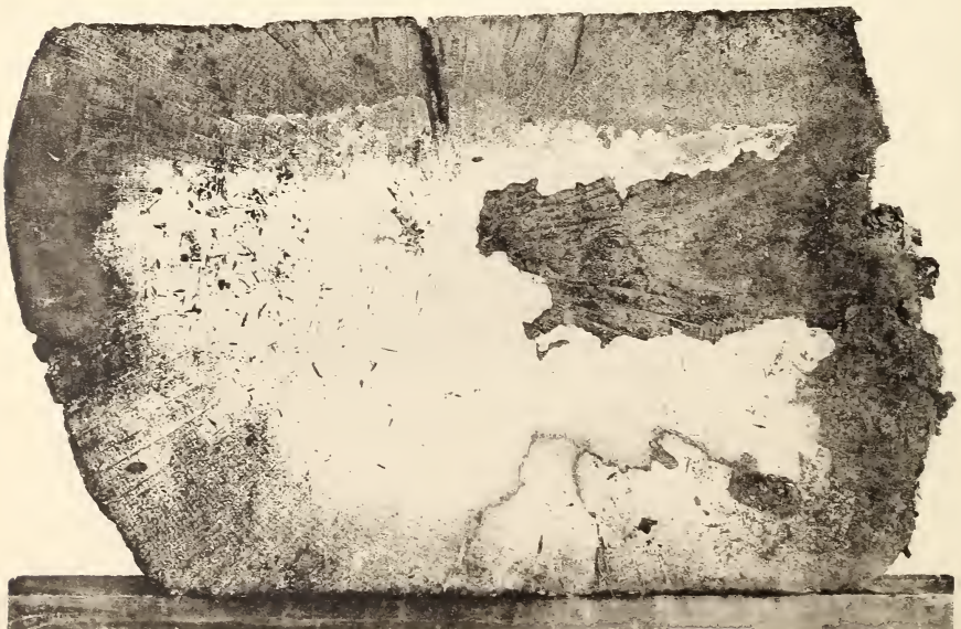
Fig. 2. White oak tie, showing growth of destructive fungus.
