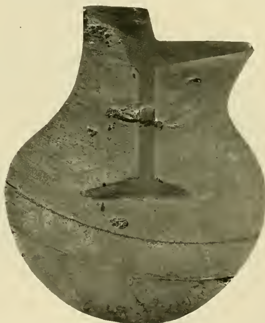
SECTION OF CAST-WELDED JOINT.
