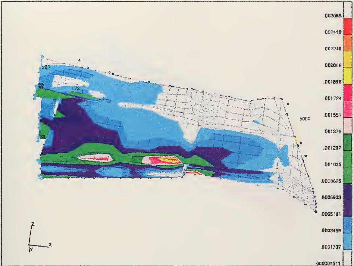
Figure 32: Vertical Strain Energy Density Fringe of Bulk-Mod Model
