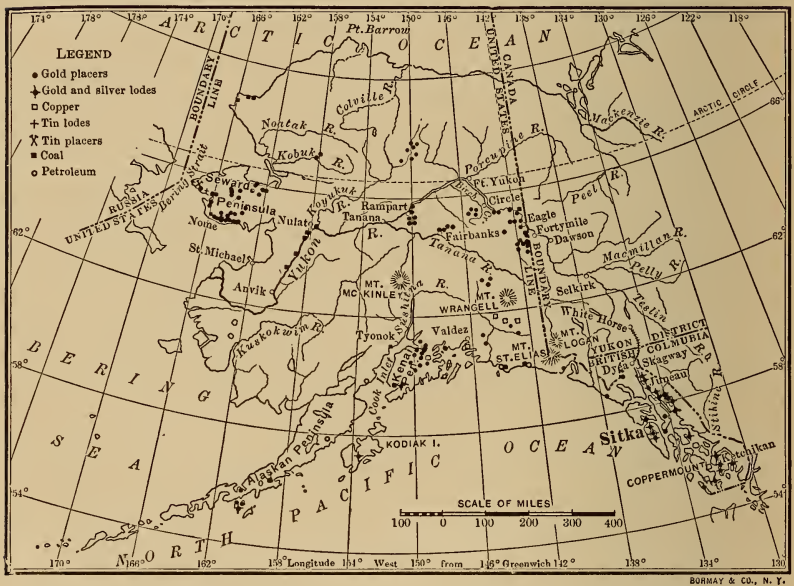
FIG. 81.—Map showing mineral deposits of Alaska as far as known. After Brooks, U. S. Geol. Surv., Bull. 259 .
