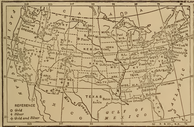
FIG. 69.—Map showing distribution of gold and silver ores in United States. Adapted from Ransome, Min. Mag. , X: 1.
