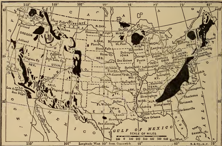
FIG. 20. — Map showing distribution of crystalline rocks (mainly granites) in United States. After Merrill. Stone for Building and Decoration.
