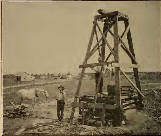
FIG. 68. — A typical hoisting outfit in the southwestern Missouri zinc region. Photo. by H. F. Bain.
