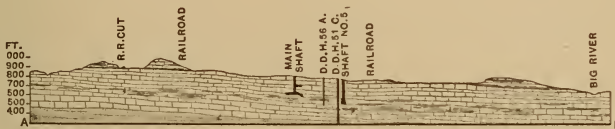
FIG. 43.—Section at Bonne Terre, Mo., showing ore disseminated through limestone.
