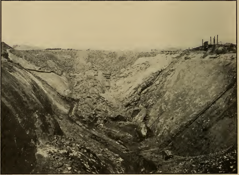
FIG. 1.—Pit working (Strippings) near Milnesville, Pa. The Mammoth seam is uncovered in bottom of pit.
