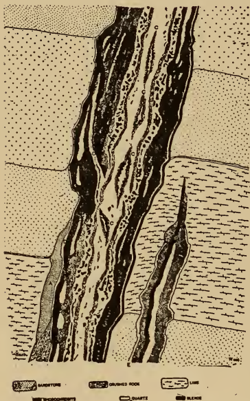
FIG. 87.—Vein filling a fault fissure, Enterprise mine, Rico, Colo. After Rickard, Amer. Inst. Min. Eng., Trans. XXVI: 927.
