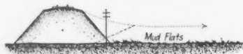
Fig. 2.—Sketch Showing Displacement of Track by Ocean Waves on the Old Colony R. R.
