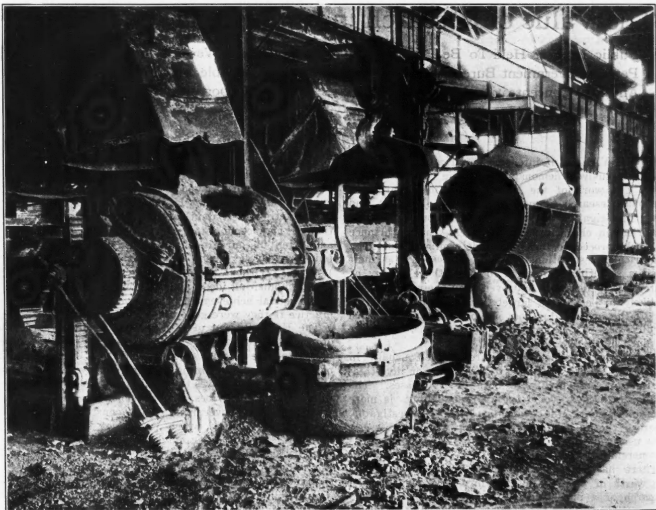
BASIC CONVERTER AND CASTING FURNACE AT THE OLD DOMINION SMELTER AT GLOBE
