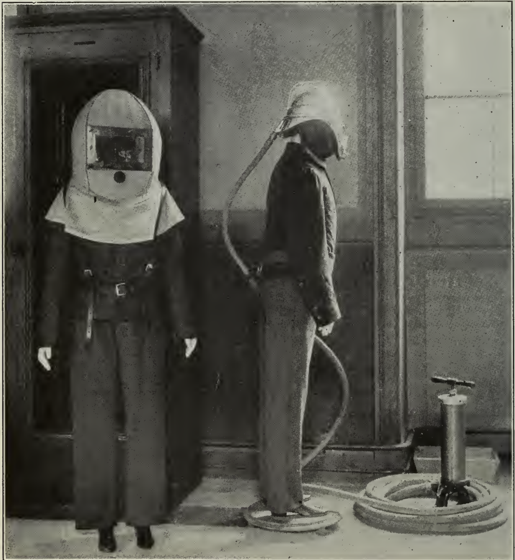
FIG. 8. RESPIRATORY HELMET, PARIS FIRE-DEPARTMENT TYPE, AND PROTECTIVE HELMET FOR SAND-BLASTERS, CASASSA SYSTEM.
