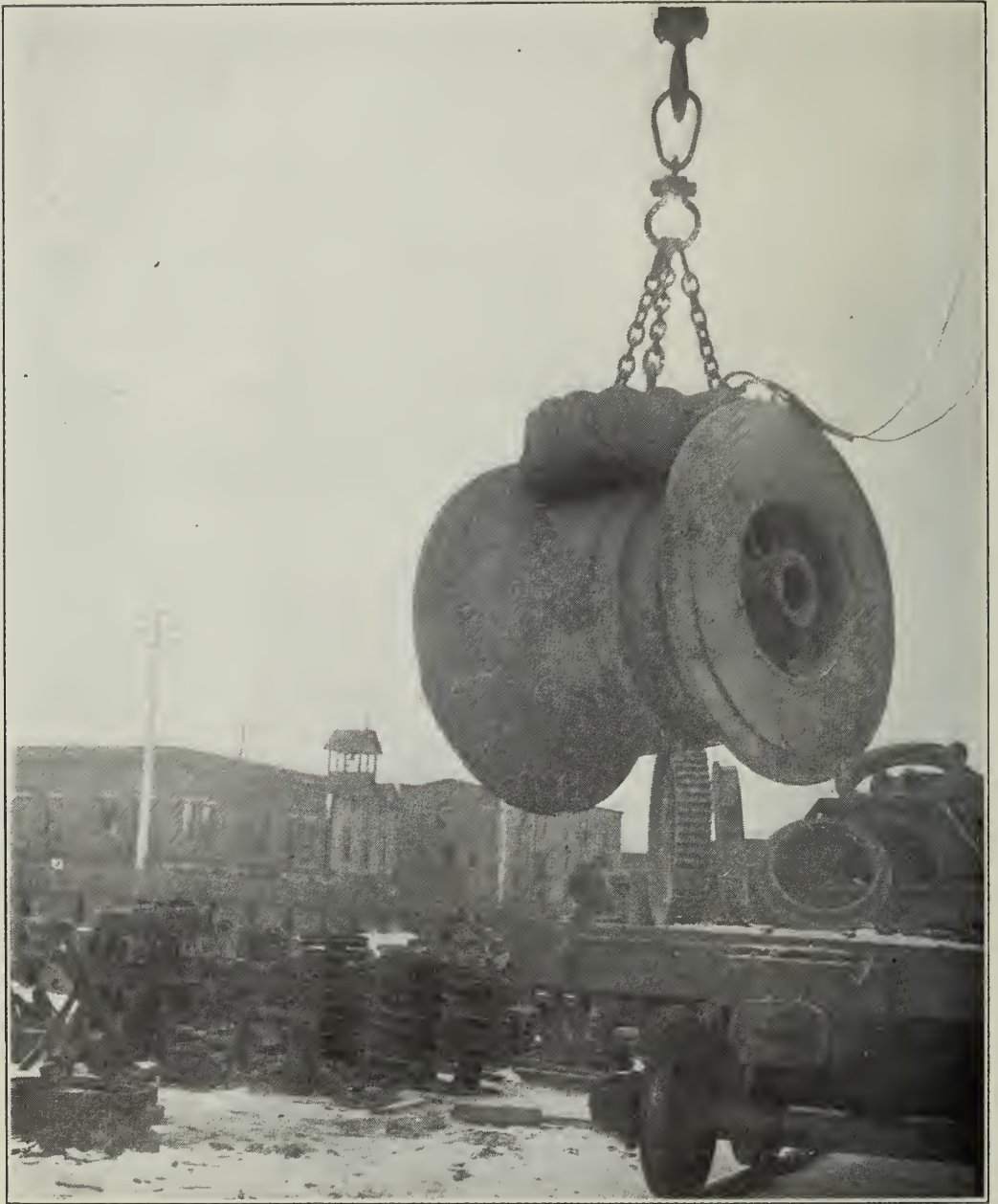
CUTLER-HAMMER LIFTING MAGNET UNLOADING CASTINGS.
