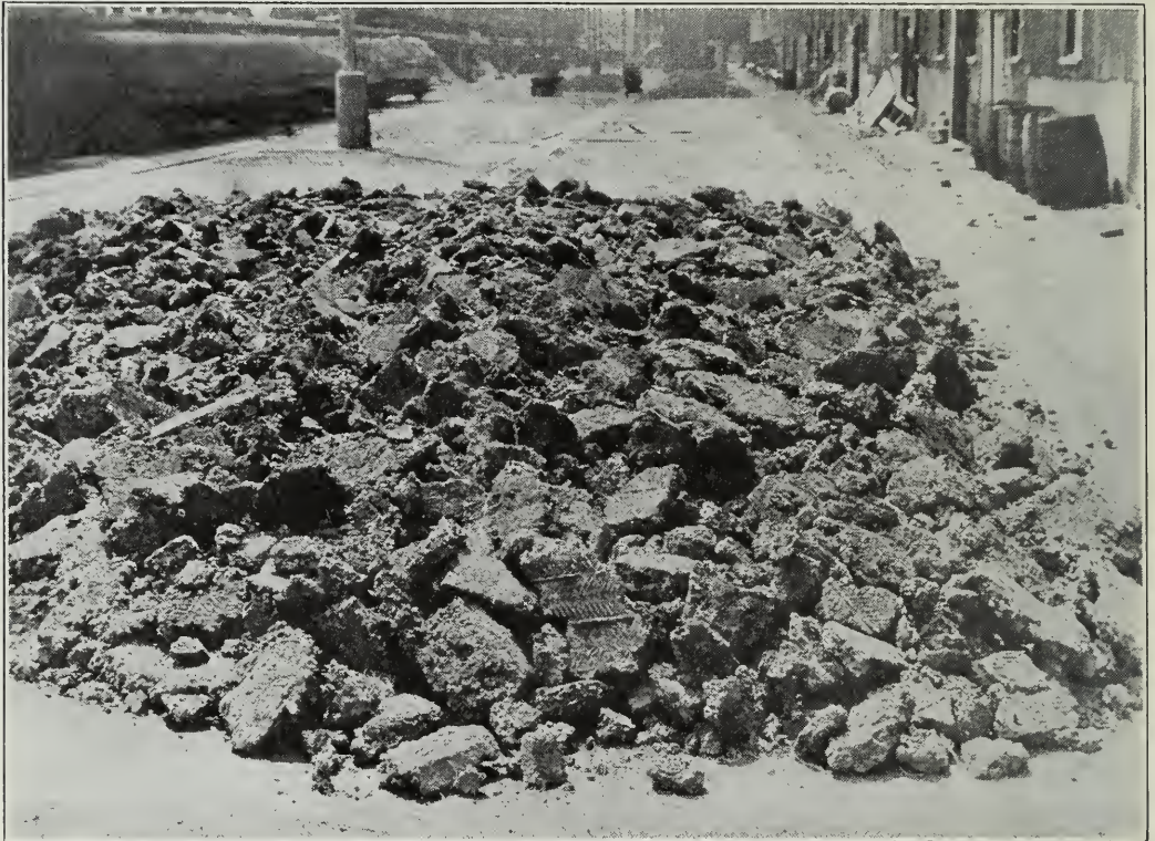
SINTER CARRYING 50 PER CENT. LEAD, MADE FROM GALENA CONCENTRATES WITHOUT LIME.
