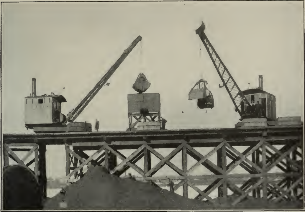
TWO LOCOMOTIVE CRANES WITH GRAB BUCKETS, UNLOADING COAL FROM BARGES TO STORAGE.
