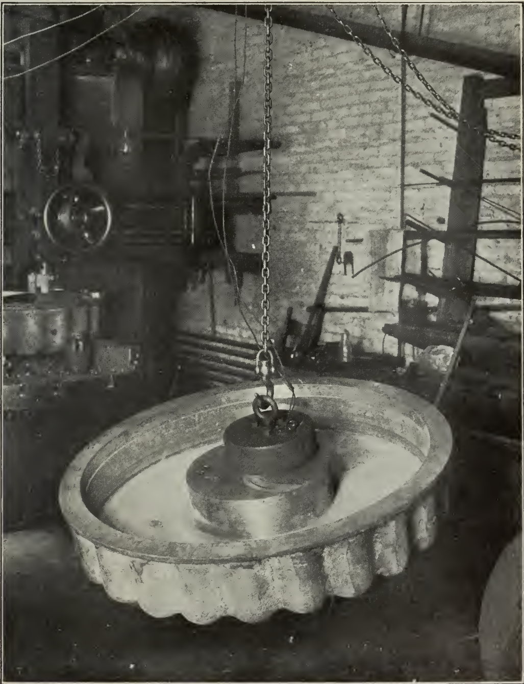
A 10-INCH CUTLER-HAMMER MAGNET LIFTING THE BODY OF A 50-INCH MAGNET. The casting, ready for insertion of the coil and coil shield, weighs about 3000 lb. and is of awkward shape to handle with slings. An apt illustration of the advantages of this mode of handling castings is thus afforded. Cutler-Hammer Mfg. Co.
