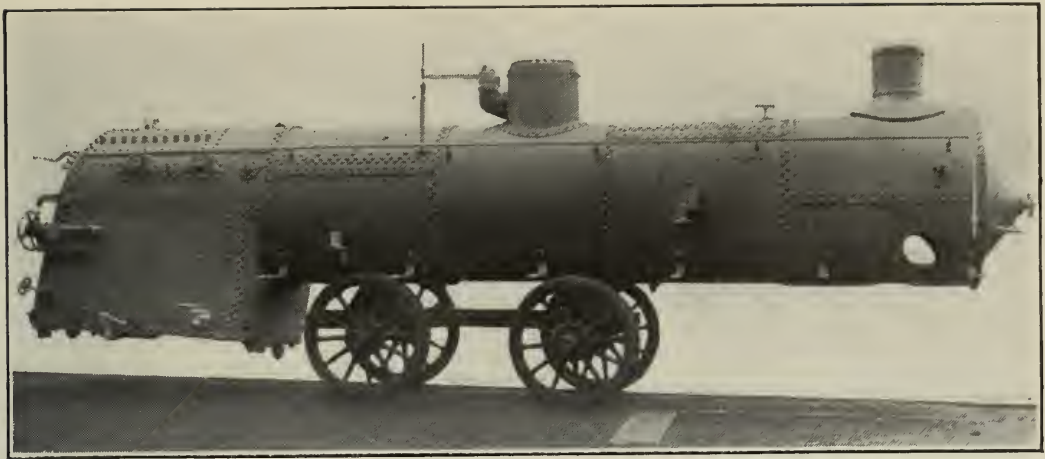
FIG. 18. WIDE-TYPE FIREBOX AND PARALLEL BOILER, APPROVED IN RECENT CONTINENTAL PRACTICE.
