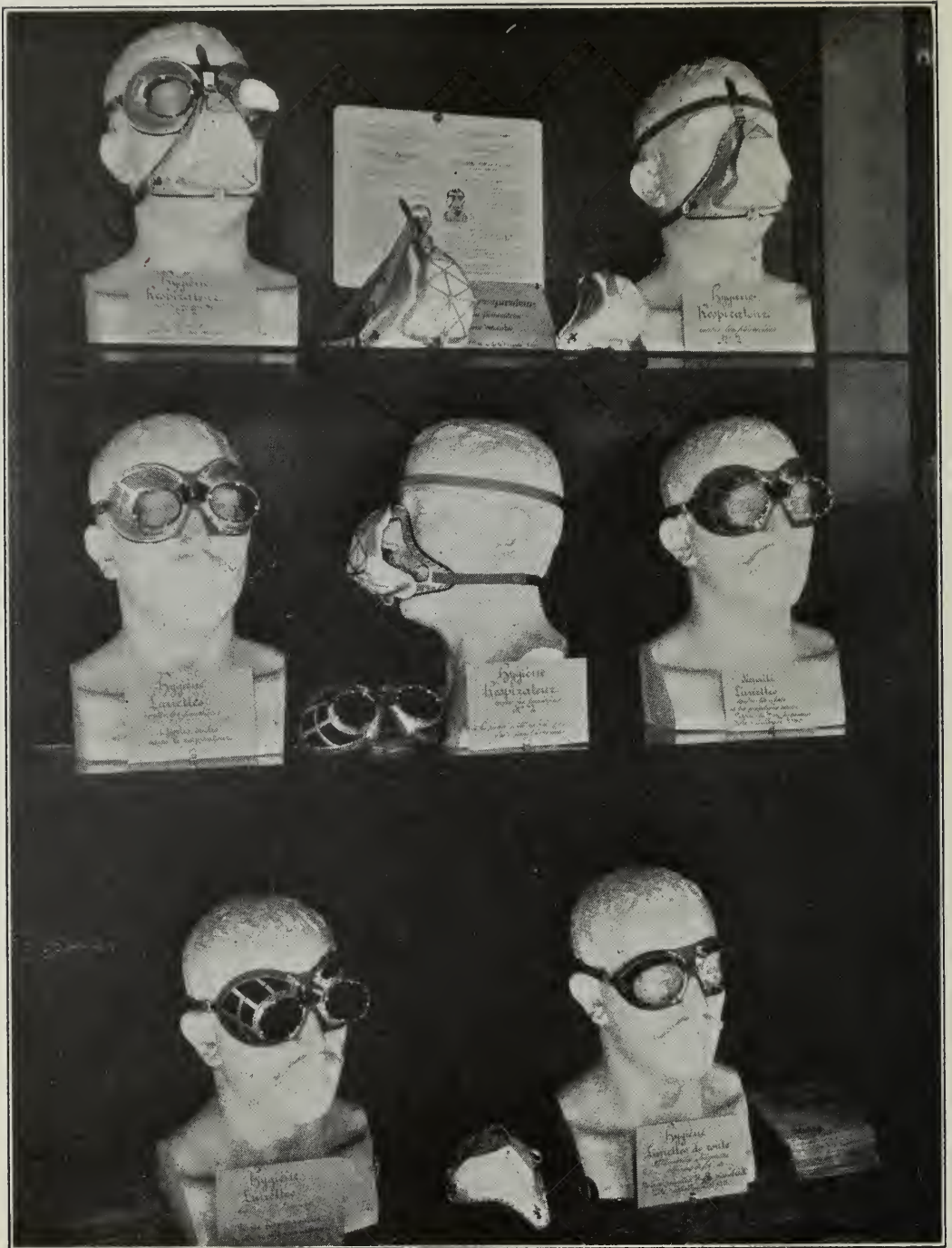
FIG. 6. PROTECTIVE SPECTACLES AND RESPIRATORY APPLIANCES FOR PROTECTION AGAINST DUST, DEVISED BY DR. DÉTOURBE.
