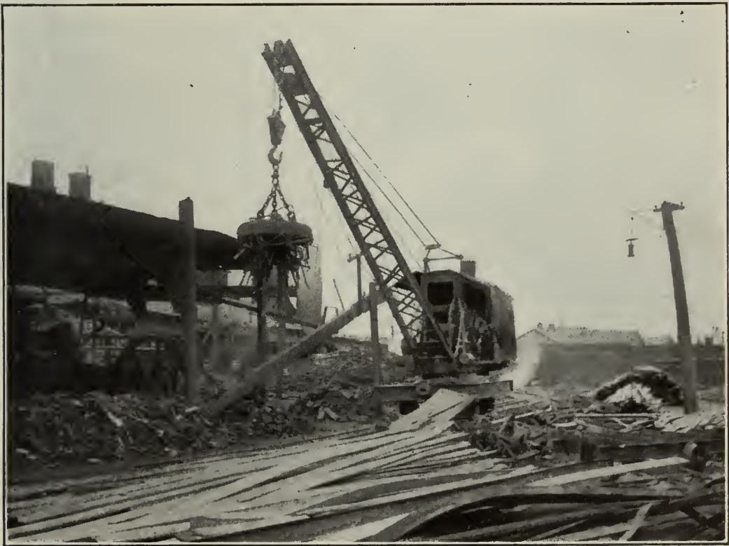
LOCOMOTIVE CRANE EQUIPPED WITH ELECTRIC LIFTING MAGNET HANDLING LOOSE SCRAP.
