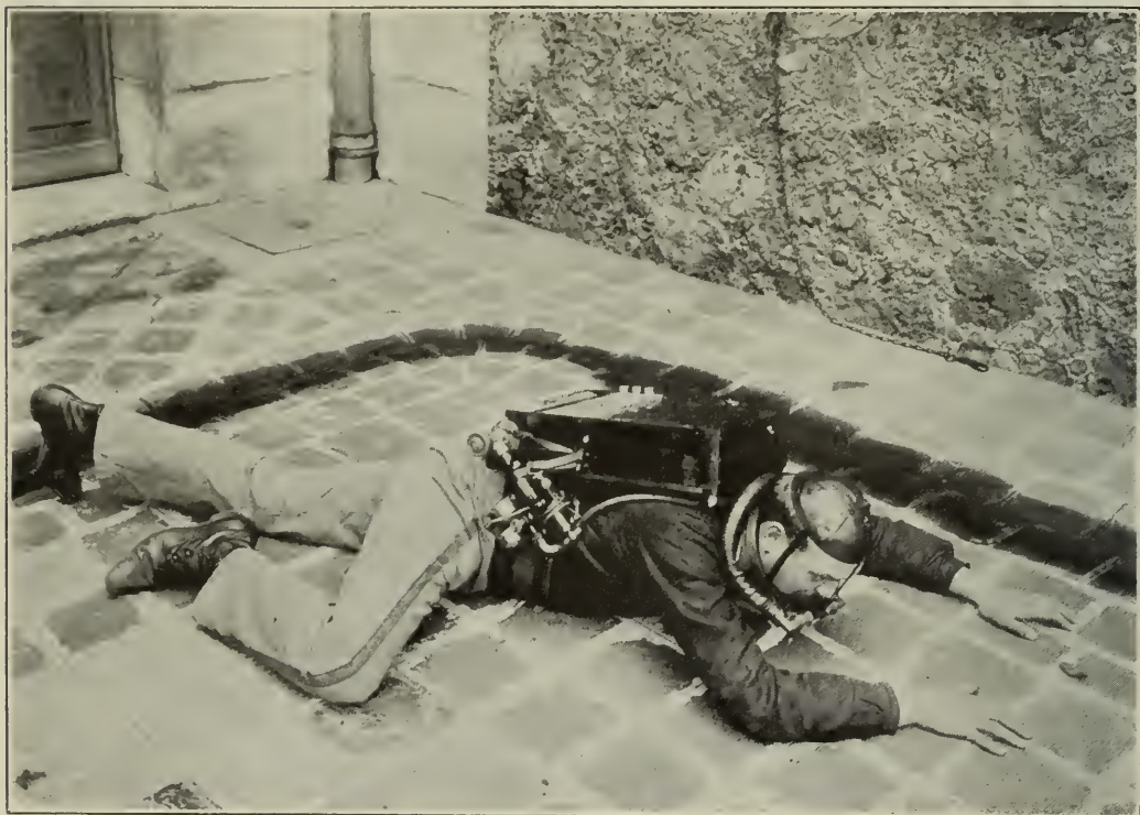
FIG. 8. TISSOT RESPIRATORY APPARATUS; SHOWING HOW THE RESCUER MAY CRAWL FLAT ON HIS STOMACH WITHOUT INCONVENIENCE.
