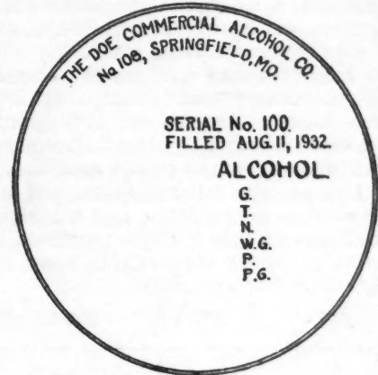
Marks on Filling or Entry Into Warehouse.
