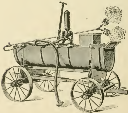
FIG. 36—Double-acting horizontal pump mounted on 250-gallon tank. A good type of outfit for medium sized commercial orchards. (Va. Agr. Exp. Sta.)
