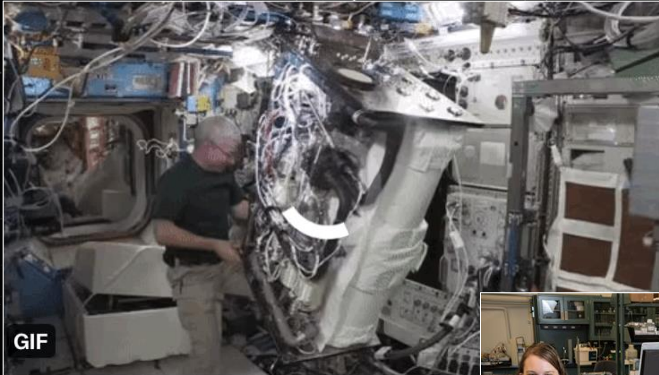
Above: Mark Van de Hai installing 4-Bed CO2 Scrubber in the US Laboratory
