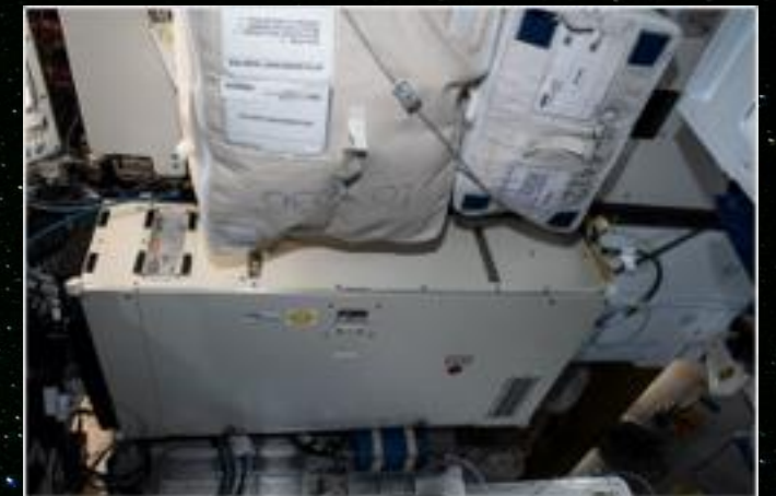
Below: Brine Processor Assembly installed in March 2021
