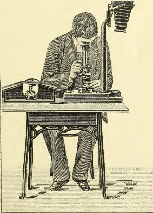
Camera swung aside to admit of adjustment of light, focusing, &c.
