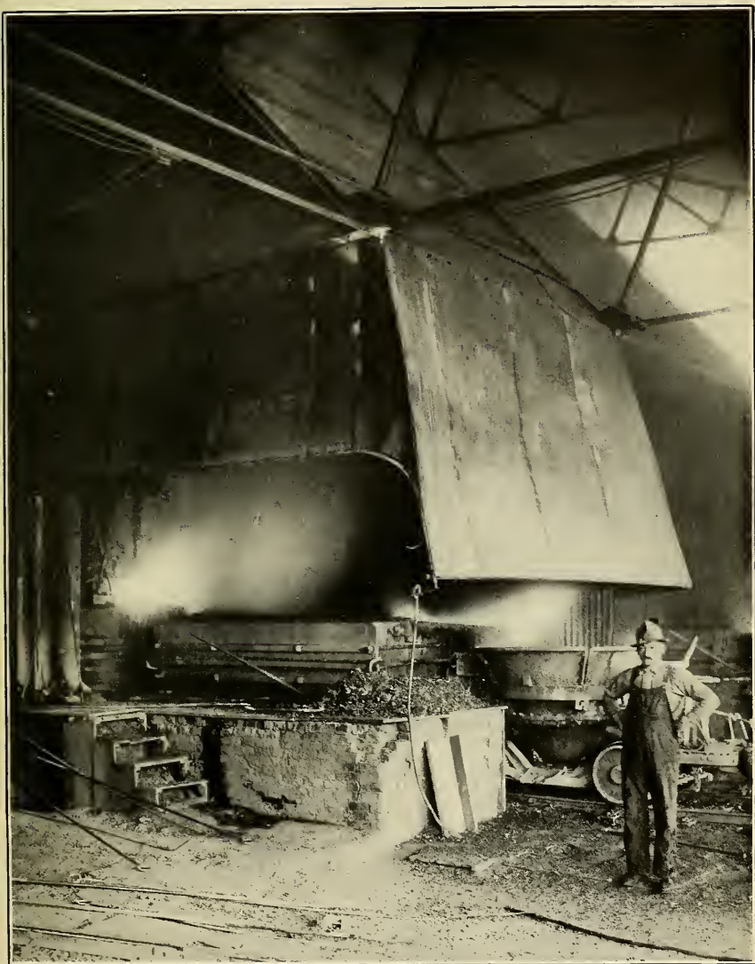
PLATE 8.—TAPPING FLOOR OF A BLAST FURNACE IN THE AMERICAN SMELTING & REFINING CO.'S PLANT AT MURRAY, UTAH.
