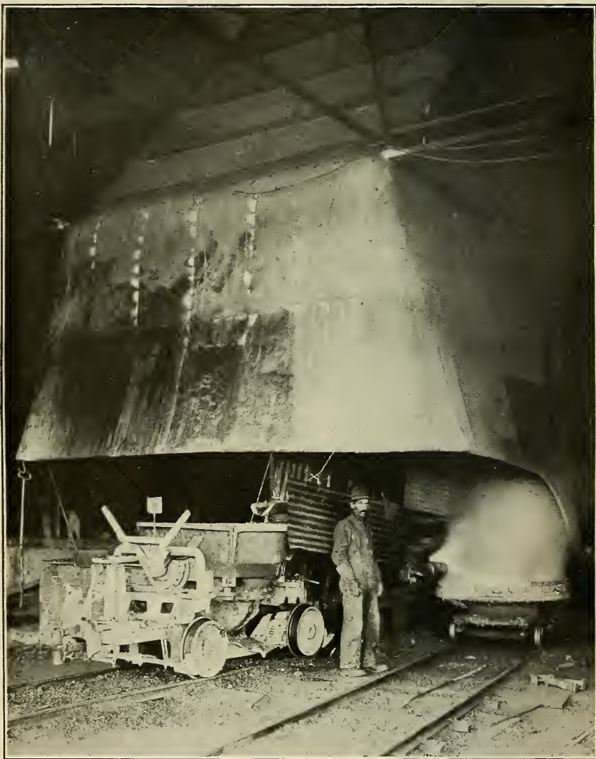
PLATE 9.—MATTE TAPPING IN THE AMERICAN SMELTING & REFINING CO.'S PLANT AT MURRAY, UTAH.
