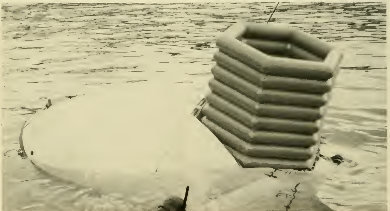
Fig. 14.15 Inflated conning tower on DEEPSTAR 4000 . (Westinghouse Corp.)
