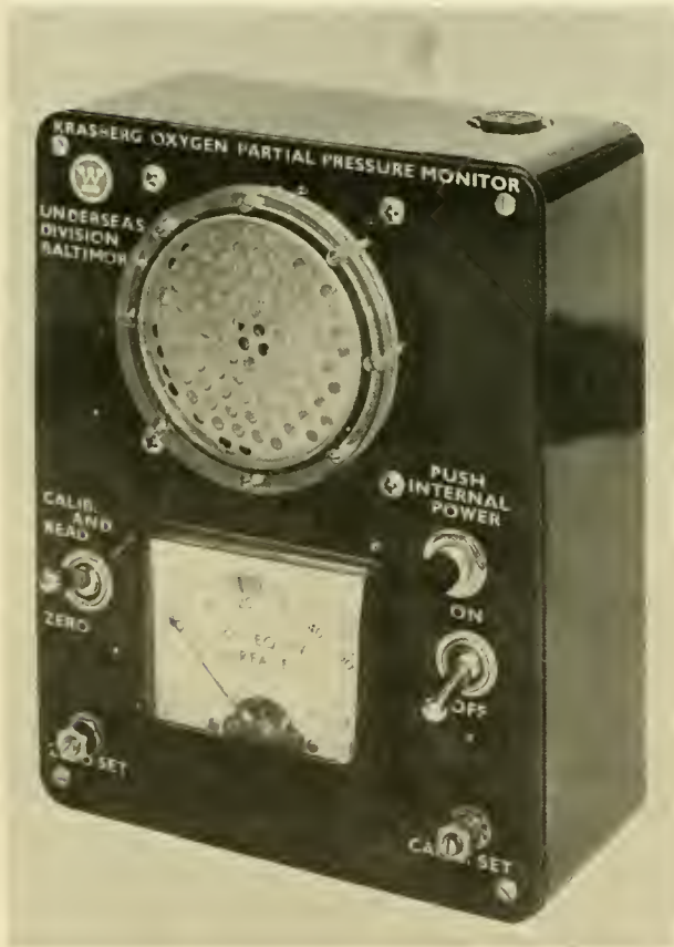
Fig. 9 14 Westinghouse-Krasberg oxygen monitor. (Mr. A. P. Ianuzzi, Naval Facilities Eng. Comm.)
