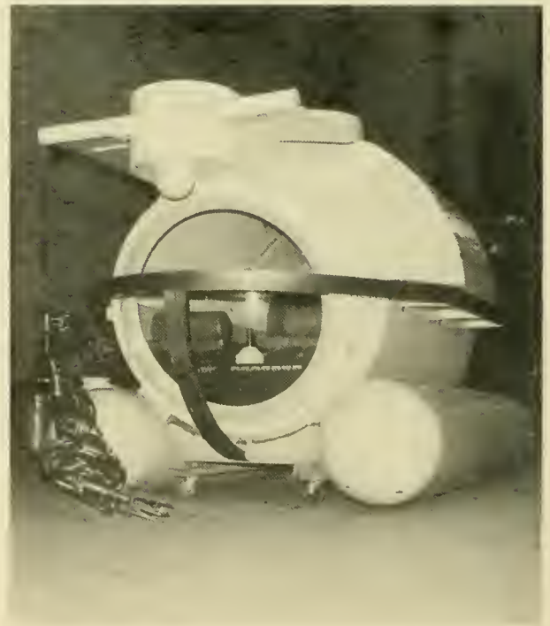
Fig. 3.31 AQUARIUS I typifies the new breed of submersibles: shallow depth, simple construction and operation and panoramic viewing. (HYCO)
