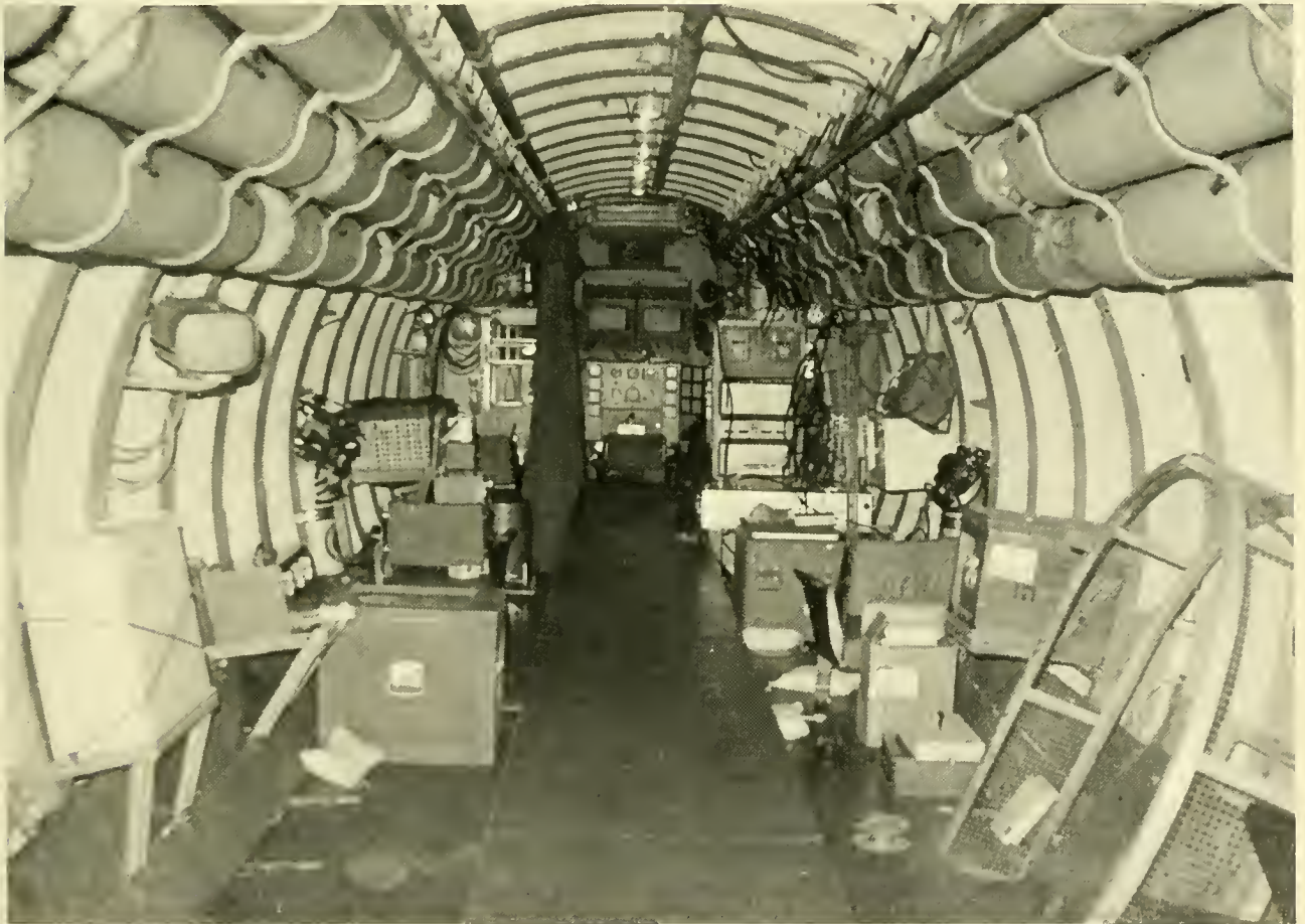
Fig 6.1 Interior of AUGUSTE PICCARD . Overhead rows of cylindrical tanks port and starboard hold a total of 842.5 cubic feet of compressed air for blowing main and variable ballast.
