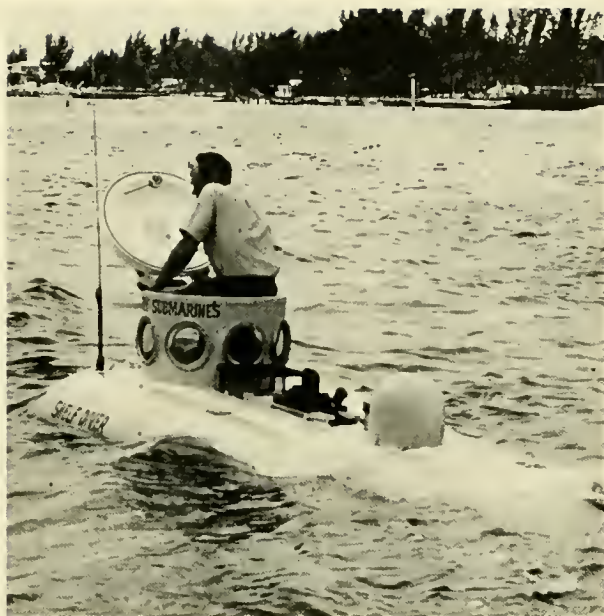
Fig. 10.22 To reduce the interfering effects of the hull on its magnetic compass, SHELF DIVER 's compass is mounted off of the conning tower in the bubble-like protrusion
