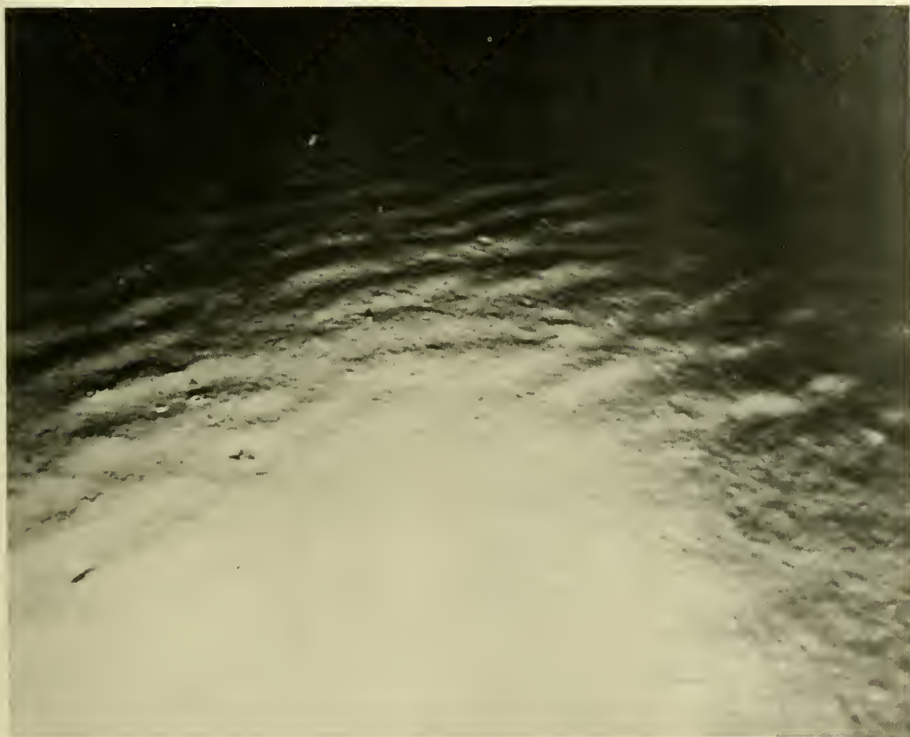
Fig. 10.7 A photograph of the sea floor taken from ALVIN. Note the overexposed region or "hot spot" and underexposed regions at the extremities. Subsequent lighting rearrangements provided more uniform exposure. (U.S. Navy)
