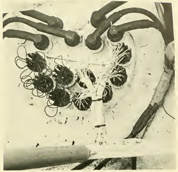
Fig. 7.20 Piccard penetrators with Marsh Marine (Vector) connectors and specially-designed main power penetrators on BEN FRANKLIN . (NAVOCEANO)
