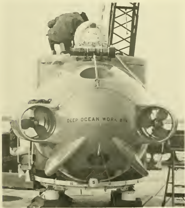
Fig. 8.4 The Ducted Propellers on DOWB provide surge and yaw thrust. The two motors are in the deck plane of the vehicle and canted outboard at angles of 15 degrees. (NAVOCEANO)
