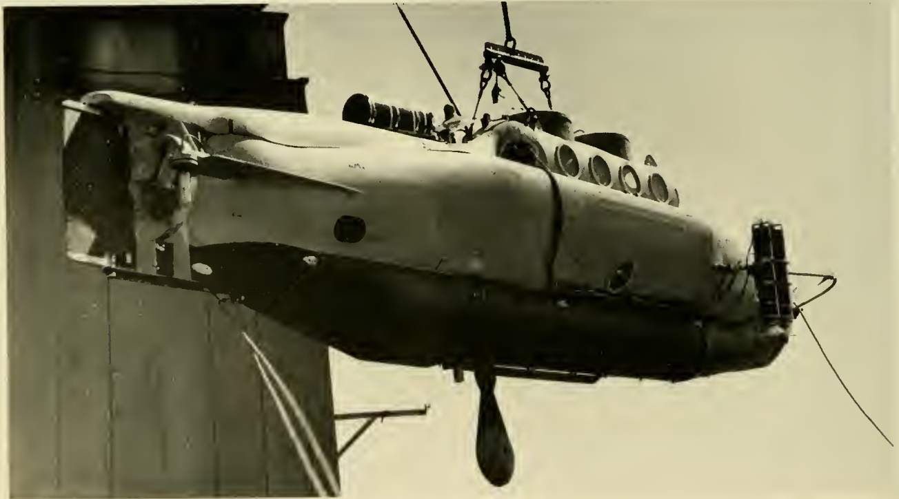
Fig. 8.9 The PC-3B is provided yaw motion by its stern rudder and pitch by plexiglass bow planes not visible here. (NAVOCEANO)
