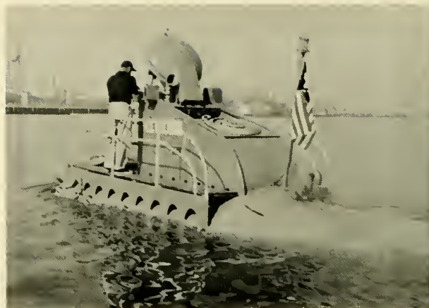
Fig. 3.8 Edmund Martine's SUBMANAUT used diesel engines for surface power and batteries when submerged. (Edmund Martine)
