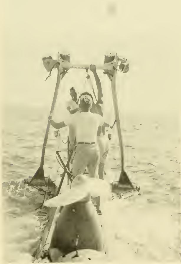
Fig. 10.8 Crewman of ALUMINAUT in the process of lowering a light boom containing four EG&G incandescent lights. (U.S. Navy)
