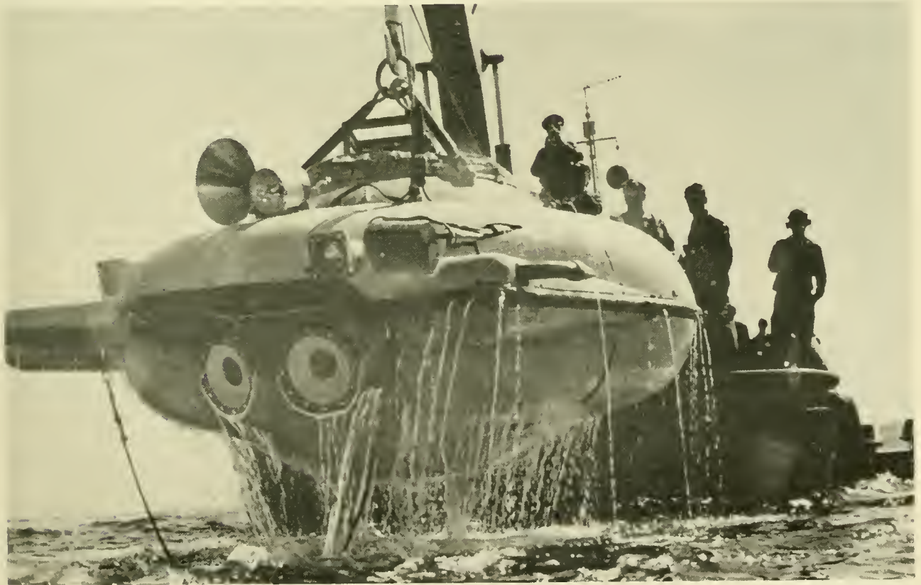
Fig. 8.7 Propulsion for SP-350 is provided by two water jets mounted port and starboard on the centerline forward. The port jet can be seen here pointing directly aft. (NAVOCEANO)
