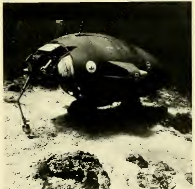
Fig. 3.19 Originally slated for 12,000 feet, DEEPSTAR 4000 represented the first Westinghouse candidate for deep diving. In its 4-year career the versatile craft would conduct over 500 dives and add significantly to our knowledge of the deep sea. (NAVOCEANO)
