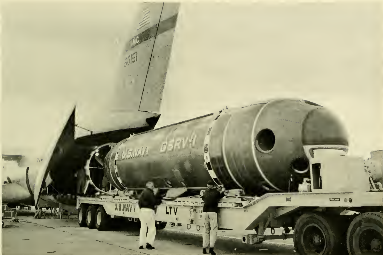
Fig 12.2 DSRV-1 entering a C-141A with mating skirt removed (U.S. NAVY)
