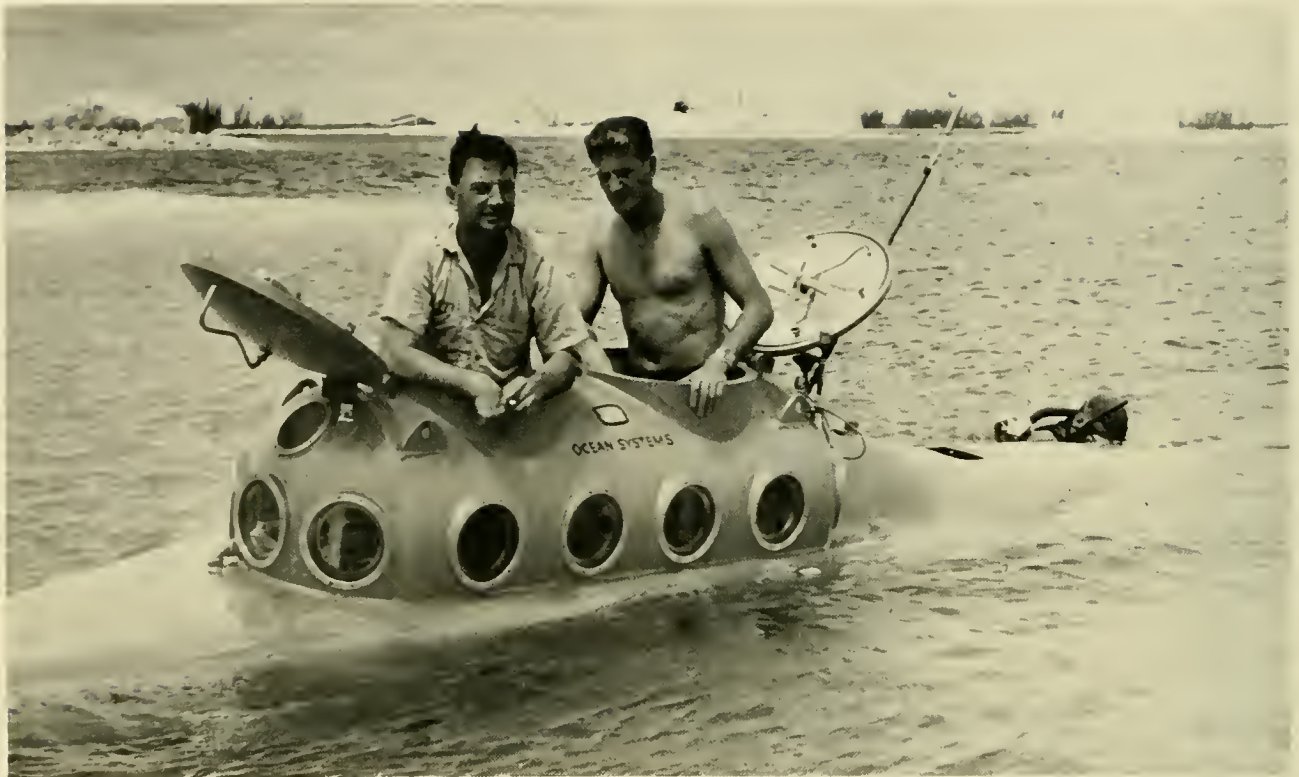
Fig. 14.14 Protection from swamping is afforded by TECHDIVER's (PC-3B) extended pressure hull (NAVOCEANO)
