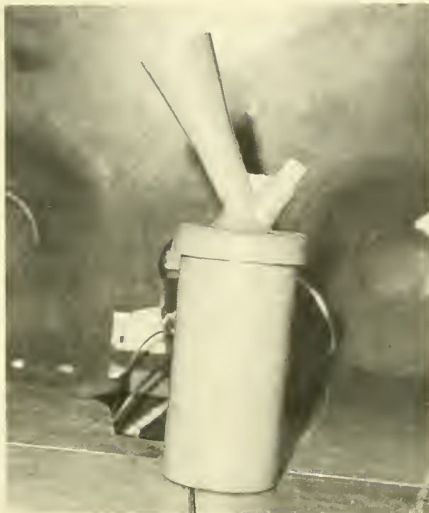
Fig. 9.7 DEEPSTAR 2000's human element range extender (HERE).
