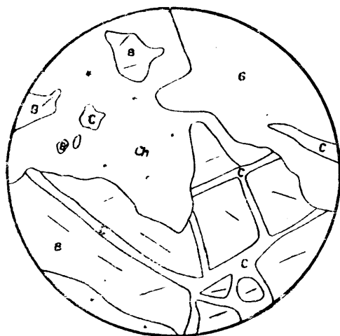
Fig. 38. Copper ore of Hsinshan, Tungchuan, Yunnan. \times 62 . Chalcopyrite contains irregular masses of bornite and covellite which replaces bornite along the fracture. G. Gangue. C. Covellite. B. Bornite. Ch. Chalcopyrite.
