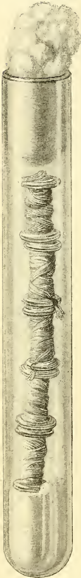
FIG. 9.—ROLLS OF STERILIZED SILK THREADS ON GLASS BOBBINS PRESERVED IN STOUT GLASS IGNITION TUBES. \frac{3}{4} ORDINARY SIZE.
