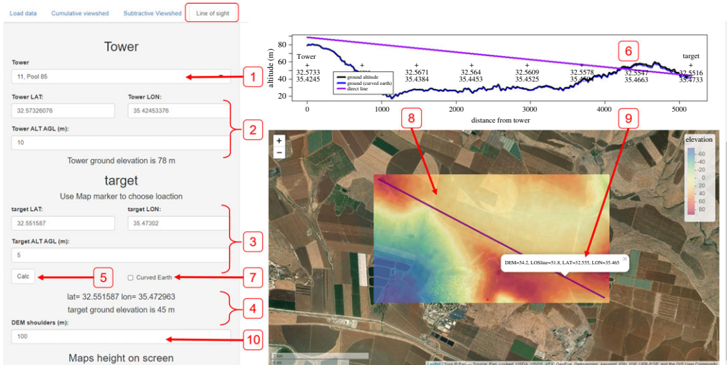
Figure 5. The ‘Line of sight’ (LOS) tab. The user may choose a tower from a drop-down list (1) or manually type its coordinates in Lat-Lon and height above ground (2). Similarly, the user may choose a target location (3) either by typing its coordinates or by pinpointing a location on the map (not shown here). The coordinates and ground elevation at the chosen target point will be displayed (4). Once the ‘Calc’ button (5) is pressed the LOS will be calculated and presented in the upper right inset (6). The direct line between the points (LOS) is green if clear and purple if obstructed. The DEM elevation profile along the LOS is presented with two lines, one excluding Earth curvature (black), and one accounting for it (blue). Over short distances the two often overlap, and the latter becomes default when chosen in a tick-box (7). The bottom right panel (8) presents a map line connecting the two points and a detailed DEM in the vicinity of the points. Coordinates are presented upon clicking any point along the line (9). The DEM area can be expanded by changing the DEM shoulder value (10).
