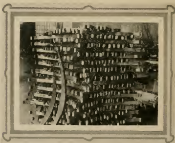
A cord of half-elliptic springs in the finishing department of plant No. 2 of The Perfection Spring Company
