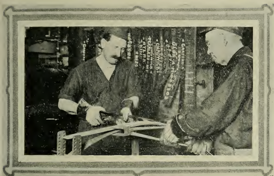
Forming spring plate over a "master" at plant No. 2 The Perfection Spring Company
