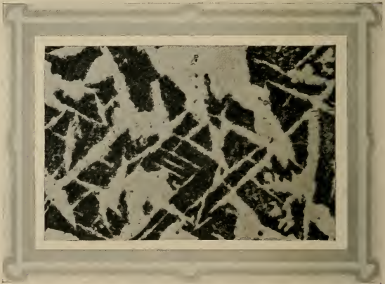
Micrograph of high carbon forging before annealing
