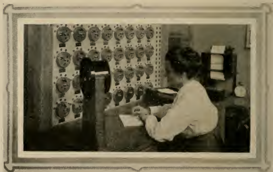
In plant No. 2 of The Perfection Spring Company, showing operator in charge of Master Pyrometer Signal System
