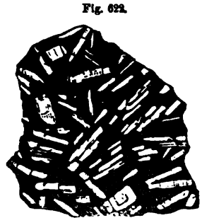
Fig. 622. Porphyry. White crystals of felspar in a dark base of hornblende and felspar.
