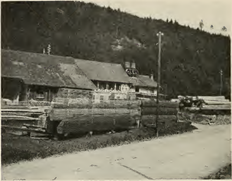
A CHARACTERISTIC SAWMILL WHERE A GREAT VARIETY OF WOOD PRODUCTS ARE MADE AND NOTHING IS ALLOWED TO GO TO WASTE. IN THE FOREGROUND, BOARDS FROM SELECT LOGS ARE PILED TOGETHER JUST AS THEY COME FROM THE SAW.
