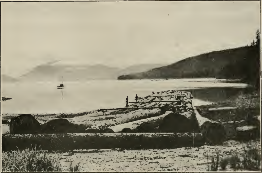
RAFT OF SITKA SPRUCE LOGS ON BEACH NEAR WRANGELL. AVERAGE DIAMETER AT THE BUTT 37 INCHES, AT THE TOP 21 INCHES. AVERAGE LENGTH, 78 FEET. CONTENTS OF RAFT APPROXIMATELY 190,000 BOARD FEET, SCRIBNER SCALE.
