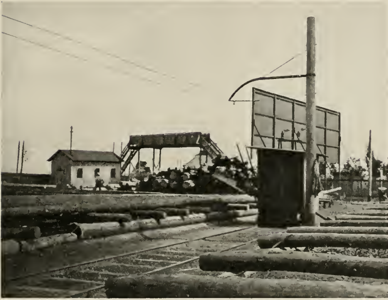
AN ELECTRIC CUT-OFF SAW USED TO CUT LONG LOGS INTO THE DESIRED LENGTHS. IT CAN BE MOVED BY OVERHEAD TROLLEY TO ANY PART OF THE ROLLWAY AND SAVES A LARGE AMOUNT OF UNNECESSARY WASTE IN TRIMMING.
