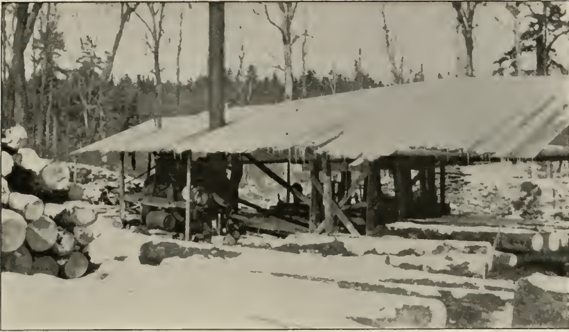
SCENE AT A PORTABLE SAWMILL USED IN NEW YORK STATE THROUGHOUT THE WINTER. NOTE SIMPLICITY OF ITS ARRANGEMENT.
