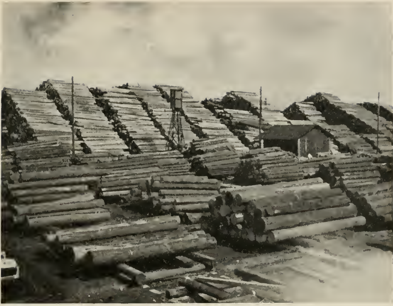
THESE LOGS ARE DECKED BY ELECTRIC MACHINERY. THIS METHOD IS USED INSTEAD OF THE AMERICAN LOG STORAGE PONDS TO HOLD THE LOGS BEFORE BEING SENT THROUGH THE MILL.
