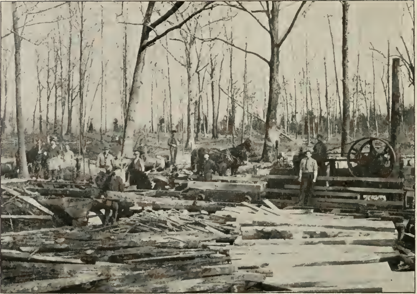
A TYPE OF A PORTABLE SAWMILL WHICH AT SLIGHT EXPENSE MAY BE SHIFTED FROM PLACE TO PLACE AS IT IS NEEDED IN CUTTING A WOODLOT.
