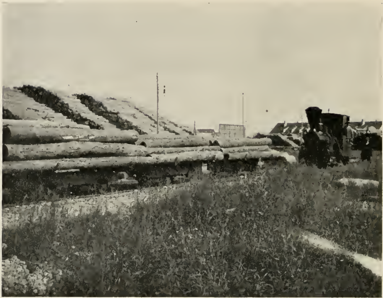
LOGS ARE USUALLY SENT INTO THE MILL ON SMALL TRUCKS RATHER THAN A JACK LADDER.
