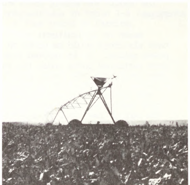
FIGURE 1-9. This pivot sprinkler rolls in a complete circle around its pivot point. Most pivots can cover about 140 acres. Sprinklers are located along the complete length of the pivot arm.
