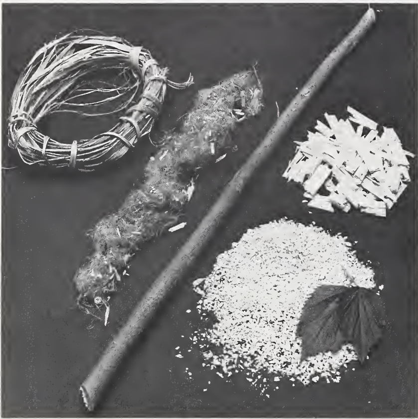
Kenaf, the bamboo-like, fiber plant native to Africa, is currently being researched for use as poultry litter. The long stalk in the center shows kenaf in its fresh-cut form. To the far left of the stalk is a circle of freshly stripped outer fiber. Next to the circle is the stuffed form of the fiber used for carpet backing. Shown to the right of the stalk is the chopped inner core being researched for use as poultry litter.
