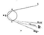
Here the ray SA (of the primary rainbow) strikes the drop at is refracted or bent to B,—is then reflected to C, where it is refracted again, and reaches the eye of the spectator.
