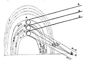
Let A, B, and C be three drops of rain; SA, SB, and SC, three rays of the sun. They are all divided into three colours, by the drops of rain on which they fall, and are reflected towards the eye at D.
