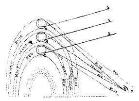
the RED (or the *least* refracted rays) of the lowest drops, all meet the eye D, and form a rainbow to the spectator.
