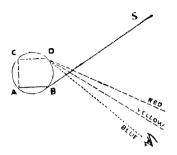
Here the ray SB (of the secondary rainbow) strikes the drop at B,—is refracted to A,—is then reflected to C,—is again reflected to D, when it is again refracted or bent, till it reaches the eye of the spectator.
