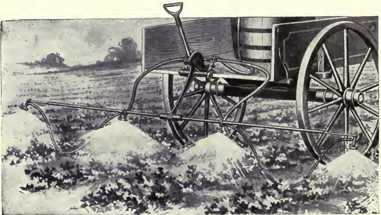
FIG. 39. - Row-spraying attachment for use with barrel pump, adjustable for various width of rows. (Deming Co.)
