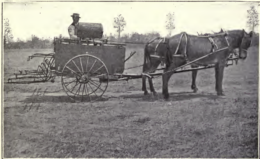
FIG. 225. — Fieldsprayer, with modifications, adapted for potato spraying by L. C. Corbett, operating at the Virginia Truck Experiment Station, Norfolk, Va.
