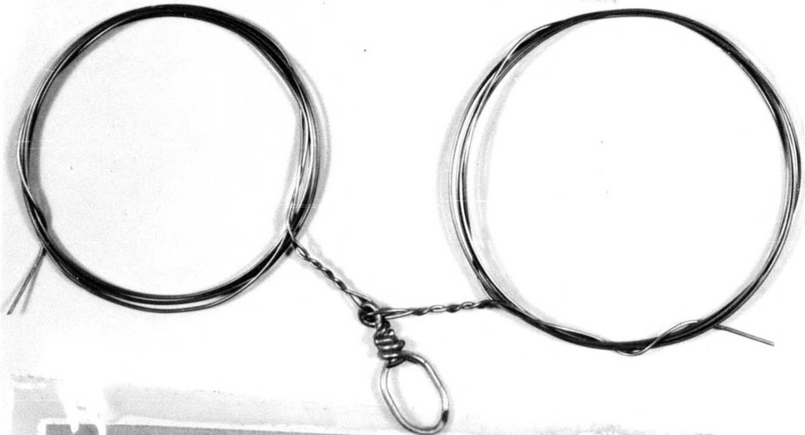
Swiveling Wire. Standard Swivel and two lengths of .033 steel safety wire
