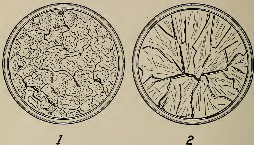
FIG. 17. (1) Puddled Clay. (2) Puddled Clay exposed to the action of freezing and thawing.
