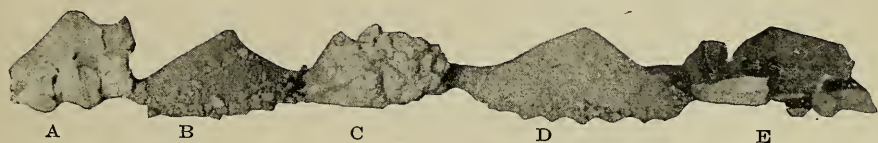
FIG. 45. Forms of lime— A—Quicklime. B—Marl. C—Water slaked lime. D—Air slaked lime. E—Limestone as marble.
