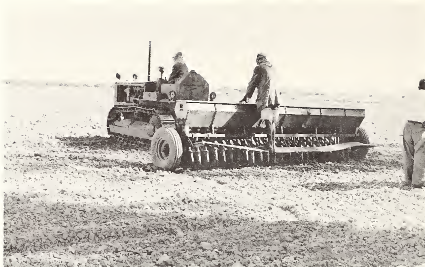
Figure 3.--A grain drill in operation on a large farm. Government of Iraq
