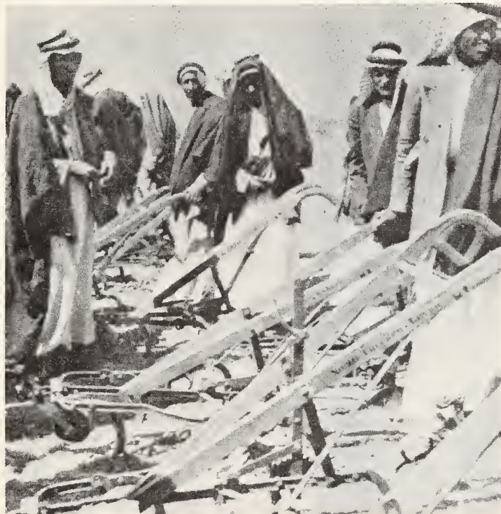
Figure 4.--Single row cultivators for use on irrigated fields where large tractor drawn equipment would be difficult to use and uneconomic.
