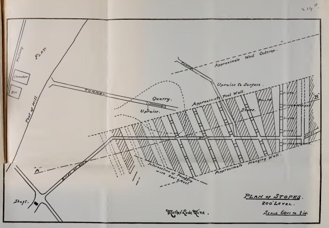
PLATE II.--Illustrating paper by Mr. Frederic Keffer, M.E., on "A Method of Mining Low Grade Ores in the Boundary Creek District."
