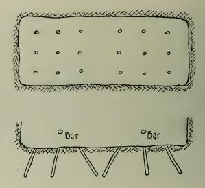
are riveted to opposite sides of the bucket near the bottom. The bucket runs on skids about 20 in. to 24 in. apart, on which strips of greased strap iron are nailed with the flat side tangent to the bucket at point of contact.
