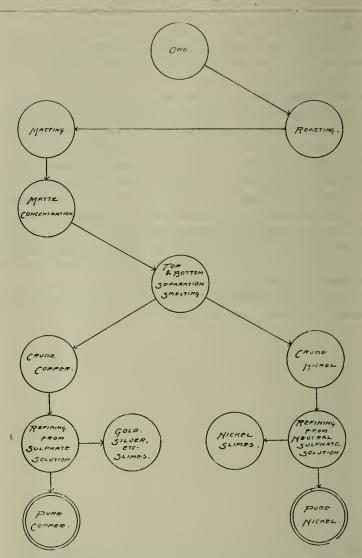
A scheme for the Production of Copper and Nickel (according to information received by writer) as proposed by Mr. Titus Ulke, for the working of Canadian Pyrrhotite Nickel Ores at the Sault Ste. Marie, Canada. From the above diagram it will be noticed the process is a refining process and uses crude metal as anode material, necessitating roasting and smelting operations together with separation smelting to the stage of obtaining a crude metal of about 90 to 95% me al centents.
