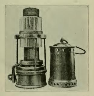
FIG. III.—Cambrian Davy Lamp for Firemen, showing glass part raised and the bonnet removed.
