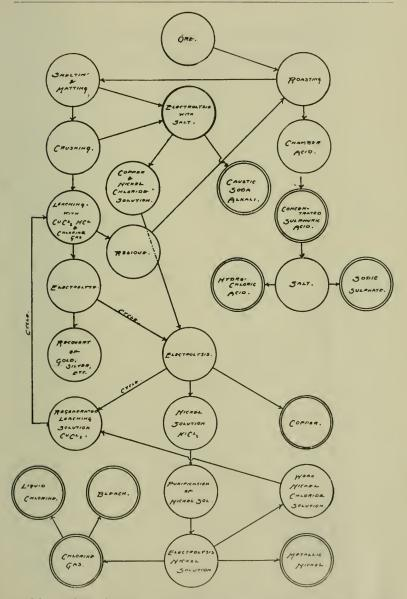
Diagram for working Chloride Solutions viz. Hoepfner Process, together with additions and improvements introduced by writer, viz. : Production of caustic (Salt Electrolysis) Liquid Chlorine, utilization of sulphur for Sulphuric Acid, Salt Cake and Muriatic Acid; also Nascent Chlorine for leaching purposes.
