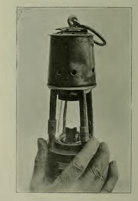
Fig. VIII.—Ashworth's patent Gray, Deputy or Fireman's Lamp. Sho mode of manipulation when testing for firedamp.
