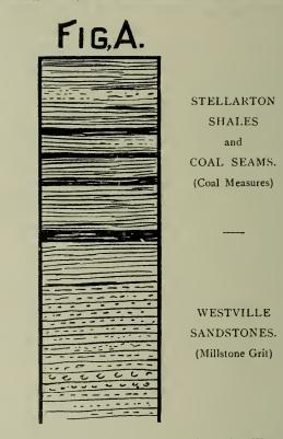
(See Figure B) — illustrating the case where the Westville and Stellarton formations are tilted at a high angle and their edges denuded. It will thus be seen that the Westville formation, with its sandstones, grits, and conglomerates, underlie unformably, and in its regular and normal position, the shales and productive coal seams and associated strata of the Stellarton formation. The block of Westville and Stellar-
