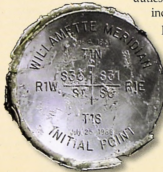
INITIAL POINT OF THE WILLAMETTE MERIDIAN GLO SURVEY. THIS STAINLESS-STEEL MARKER IS SET IN A STONE OBELISK KNOWN AS THE WILLAMETTE STONE AND IS LOCATED WITHIN WILLAMETTE STONE STATE HERITAGE AREA NEAR DOWNTOWN PORTLAND. COURTESY OF THE BLM AND THE OREGON PARKS & RECREATION DEPARTMENT.
