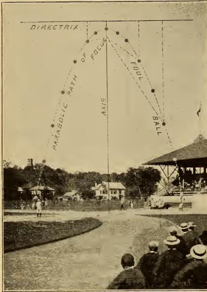
A Projectile's Path is a Parabola (From an Instantaneous Photograph by Lovell)
