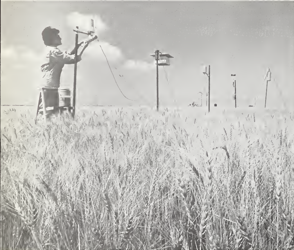
ARS soil scientist Jean Steiner checks instrumentation used for evapotranspiration research on dryland wheat. Precise field measurements help researchers develop cropping systems with improved water-use efficiency. (0686X710-1)
