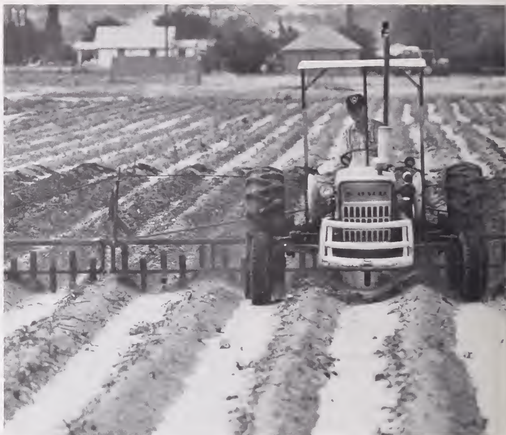
Fifty years old but still effective against wind erosion on sandy soil is the "West Texas sandfighter." As tines on the machine cut through wet soil, they throw up clods that are too big to blow away. Clods on a soil's surface can cut erosion rates by 75 to 80 percent. (0686X693-21)
