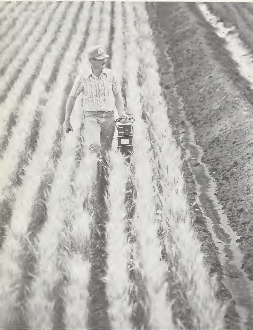
Water content of soil below bench terraces is measured periodically by Larry Fulton, ARS technician at Bushland, TX. Aim of the work is to develop better cropping and terracing systems that conserve water, increase yields, and protect soil from erosion. (0686X711-11)
