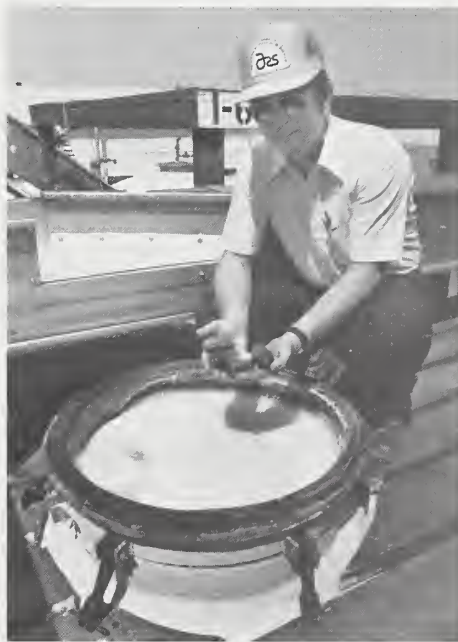
Above: Fleming at top of closed type of pickling tank which has a 30-inch diameter port through which the tank is filled and emptied. (0686X750-24)
