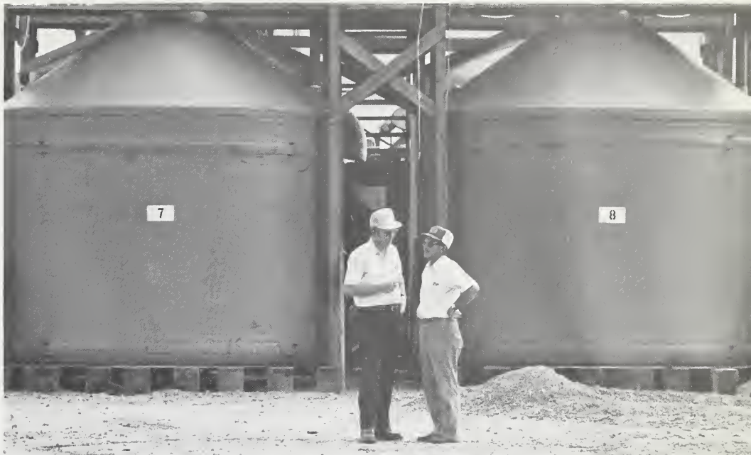
Food technologist Henry Fleming (left) and cooperating North Carolina State University scientist Ervin Humphries in front of experimental closed-top pickling tanks at the Mt. Olive Pickle Company. (0686X749-15)
