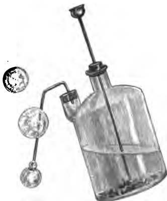
FIG. 122.—HYDROGEN BUBBLES, ILLUSTRATING PRINCIPLE OF BALLOON.
