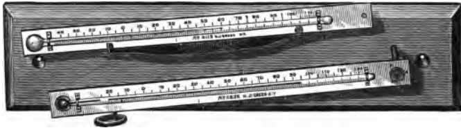
FIG. 129.—SET OF MAXIMUM AND MINIMUM THERMOMETERS. (LATEST U. S. SIGNAL SERVICE PATTERN.)
