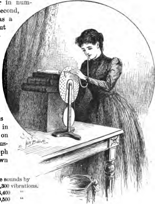
FIG. 289.—THE SIMPLE SIREN : RISE OF PITCH WITH NUM- BER OF VIBRATIONS.
