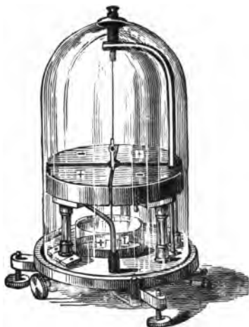
FIG. 377.—THE QUADRANT ELECTROMETER.
