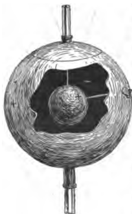
FIG. 343.—SPHERICAL CONDUCTOR, WITH INCLOSED ELECTRIFIED BALL.
