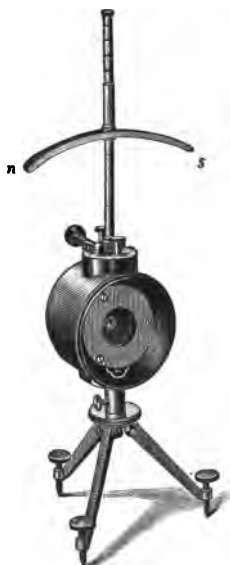
FIG. 352.—THE MIRROR GALVANOMETER.
