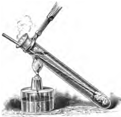
FIG. 150.—WATER A NON-CONDUCTOR.
