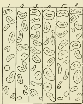
FIG. 24. Brazilian Cotton. Sections to scale \frac{1}{1000} inch between parallel lines.
