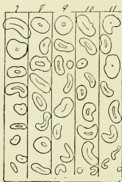
FIG. 36. Indian Cotton. Sections to scale \frac{1}{1000} inch between parallel lines.
