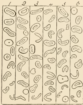
FIG. 15. American Cotton Fibres, sections to scale \frac{1}{1000} inch between parallel lines.
