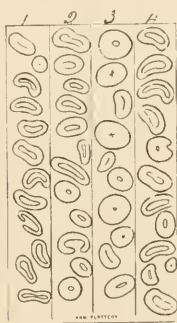
FIG. 30. Brown Egyptian Cotton. Sectional views to scale \frac{1}{1000} inch between parallel lines.
