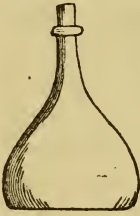
FLORENCE FLASK, used in generating chlorine gas.
