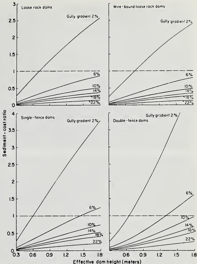
fence-type structures. The ratios remain smaller than 1.0 on all gradients larger than 5 percent for treatments with loose-rock and wire-bound loose-rock dams, and on gradients larger than 7 and 9 percent for treatments with single-fence and double-fence dams, respectively.
