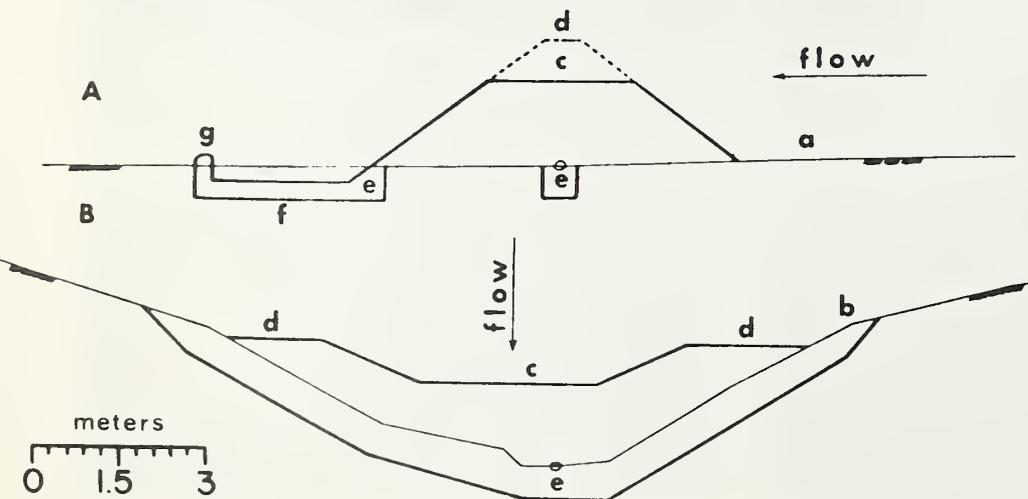
Figure 12.—Construction plans for a loose-rock check dam.
