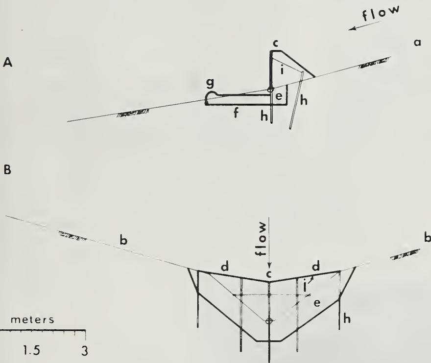
Figure 14.—Construction plans for a single-fence rock check dam.
