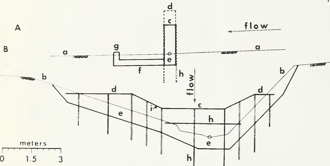
Figure 16.—Construction plans for a double-fence rock check dam.
