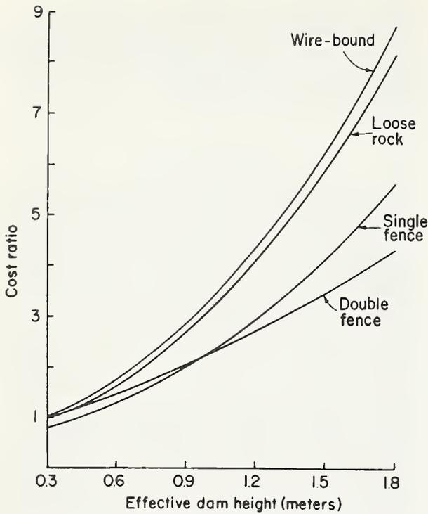
Figure 29.—Installation cost of four different types of check dams as a function of effective dam height. The cost ratio is the cost of a dam related to the cost of a loose-rock dam, 0.3-m-high, built with angular rock.
