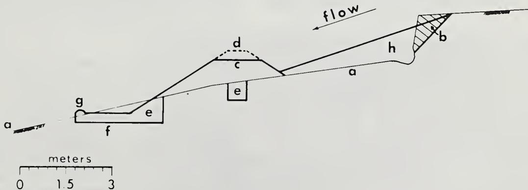
Figure 18.—Construction plan for a gully headcut control with a loose-rock check dam. The section of the structure is parallel to the centerline of the gully. a = original gully bottom; b = excavated area of headcut wall; c = spillway; d = crest of freeboard; e = excavation for key; f = excavation for apron; g = end sill; h = rock fill.
