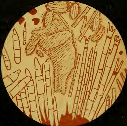
Fig. 12.—Banded rocks containing well-developed Anthophyllite crystals. Porthallow.
