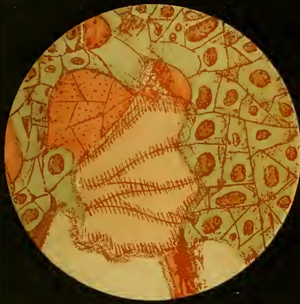
Fig. 1.—Enstatite and Olivine, Serpentine after Olivine. South of Coverack.
