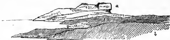
FIG. 7. SKETCH OF OVERLAP OF CRETACEOUS SANDSTONES ON TRIASSIC ARGILLITES. a. Cretaceous sandstones. b. Triassic argillites.
