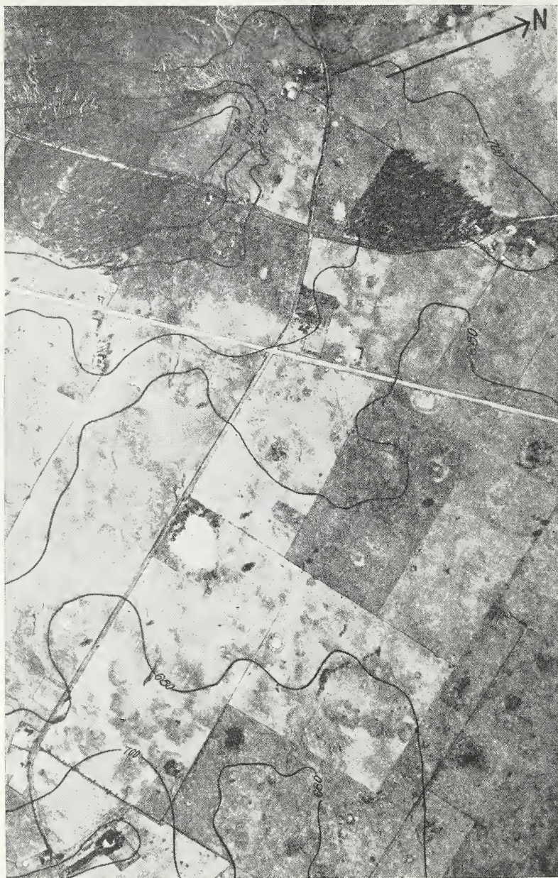
FIGURE 18.—Vertical airplane photograph of a part of the Irvington area, with contours added. The west side of the wooded knob is severely gullied. In the lowland there are many basins, some of them ponded. There are also many cistern sinks, which appear as small black specks. Shallow gullies are discernible throughout the area. The dark splotches in the lighter shaded fields represent eroded areas on basin slopes; the red subsoil photographs black.
