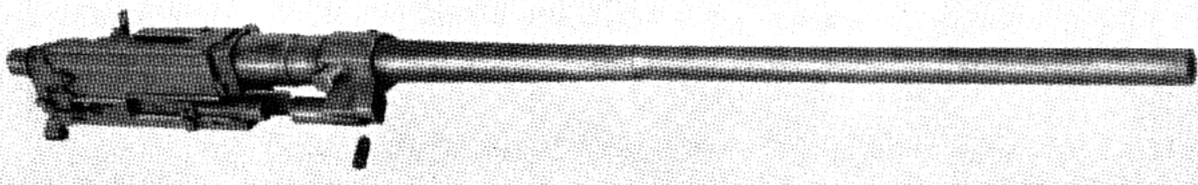
Figure 24-13. Third version of Krieghoff Experimental 20-mm Aircraft Cannon.
