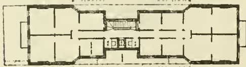
A typical floor plan of the "dumb-bell" tenement, so called, lawful up to 1901, all the interior rooms of which are lighted and ventilated on a narrow air shaft only 2' 4" in width; in which there is no separate water-closet accommodations for the different apartments and no bathing facilities.
