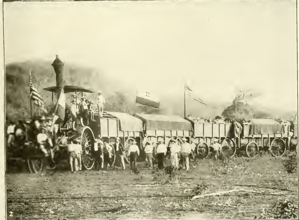
1. A 110 horse power Traction Engine hauling lumber in the Sierra Nevada Mountains. 2. Traction Engine hauling war material for the Nicaraguan government.
