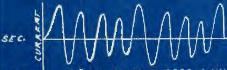
REGULAR RADIO FREQUENCY IMPULSE EXCITATION OF ANTENNA
