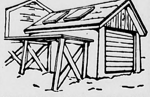
Manure Shed at Maine Station—Note the Walk, Trap-Doors in Roof, Plank End and Removable Gable.
