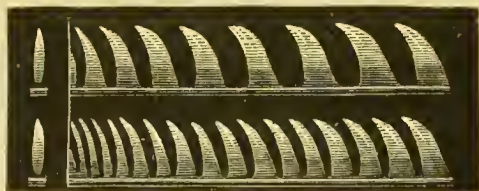
FIG. 417.—Flame picture of two organ pipes sounding an octave. It will be observed that the teeth are in the ratio of 2:1. The erect figures to the left are reflections from a small stationary mirror, for purposes of comparison.
