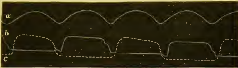
FIG. 450.—Tracings obtained from a man in the act of running. a , vertical oscillations of the body; b , impact and rise of the right foot; c , impact and rise of the left foot. When the foot presses on the ground the curve descends, it remains straight so long as the sole touches the ground, and it ascends as the sole leaves the ground. The upper horizontal part of the curve represents the time the foot remains in the air.
