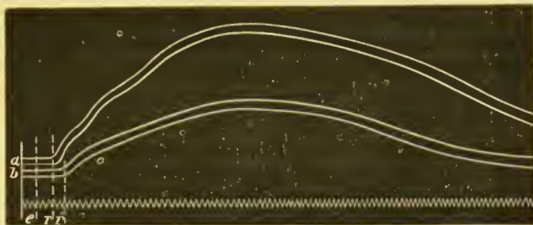
FIG. 236.—Chronograph=250 vibs. per sec. e , nerve excited far from muscle; r , near muscle; a and b , two separate experiments. The rapidity of the nerve current in the motor nerves of man has been measured by irritating the ulnar nerve at the wrist and near the elbow, the thumb being in connection with the recording apparatus.
