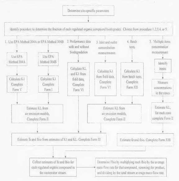
Figure 1. ALTERNATIVE EXPERIMENTAL METHODS FOR DETERMINING THE FRACTION OF ORGANIC COMPOUND BIODEGRADED (Fbio) IN A BIOLOGICAL TREATMENT UNIT Federal Register/Vol. 65, No. 13/Thursday, January 20, 2000/Proposed Rules
