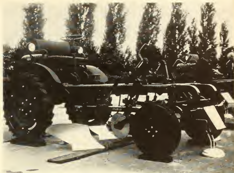
Self-propelled chassis for mounting various farm implements. Most Soviet machines are heavier than ours.
