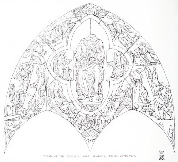
mark out the spaces to be filled by them, no joint in any case cutting through a figure. This shows that the designer of the tympanum must have been thoroughly in sympathy with the construction, even if he may not have been the constructor himself.
